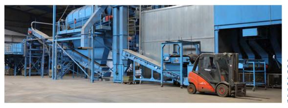
At our Lustadt site we have a mechanical processing system for small electrical devices and sophisticated composite materials. Our capacity for the sorting and separation of metals and plastics amounts to 50,000 tonnes per year.
